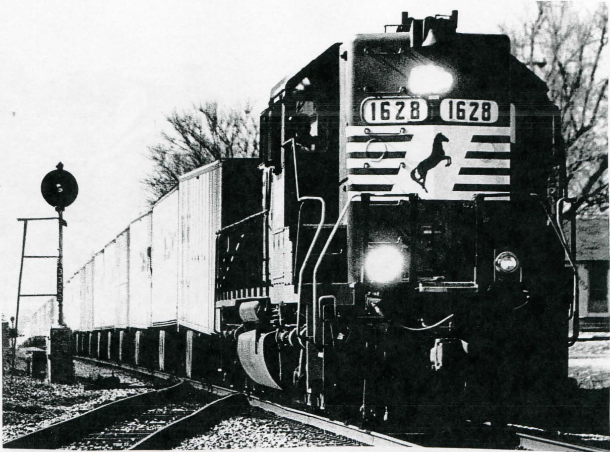
A SD40-2 heads a fast-moving Roadrailer train on the NS main eastbound through Philo in 1996.
