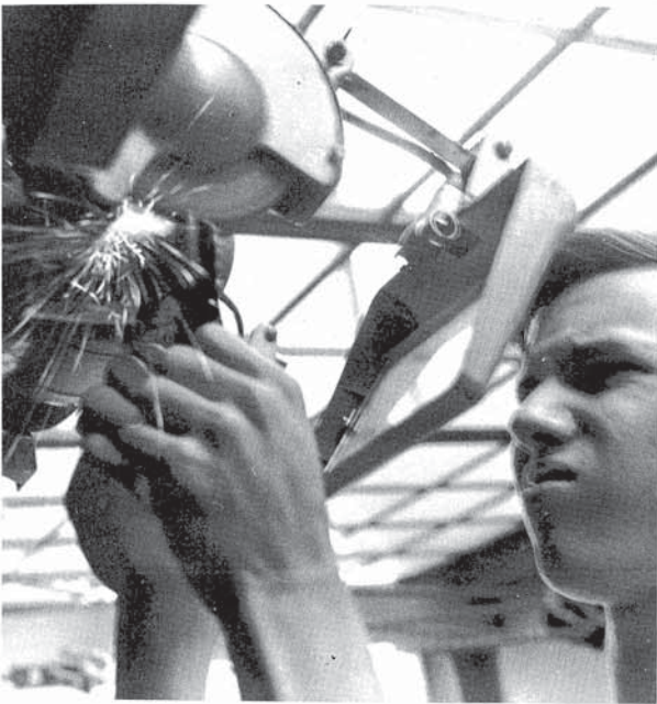
WORKING through a shield for protection from flying sparks, Mike Apperson grinds a tool bit in his metal shop class.
